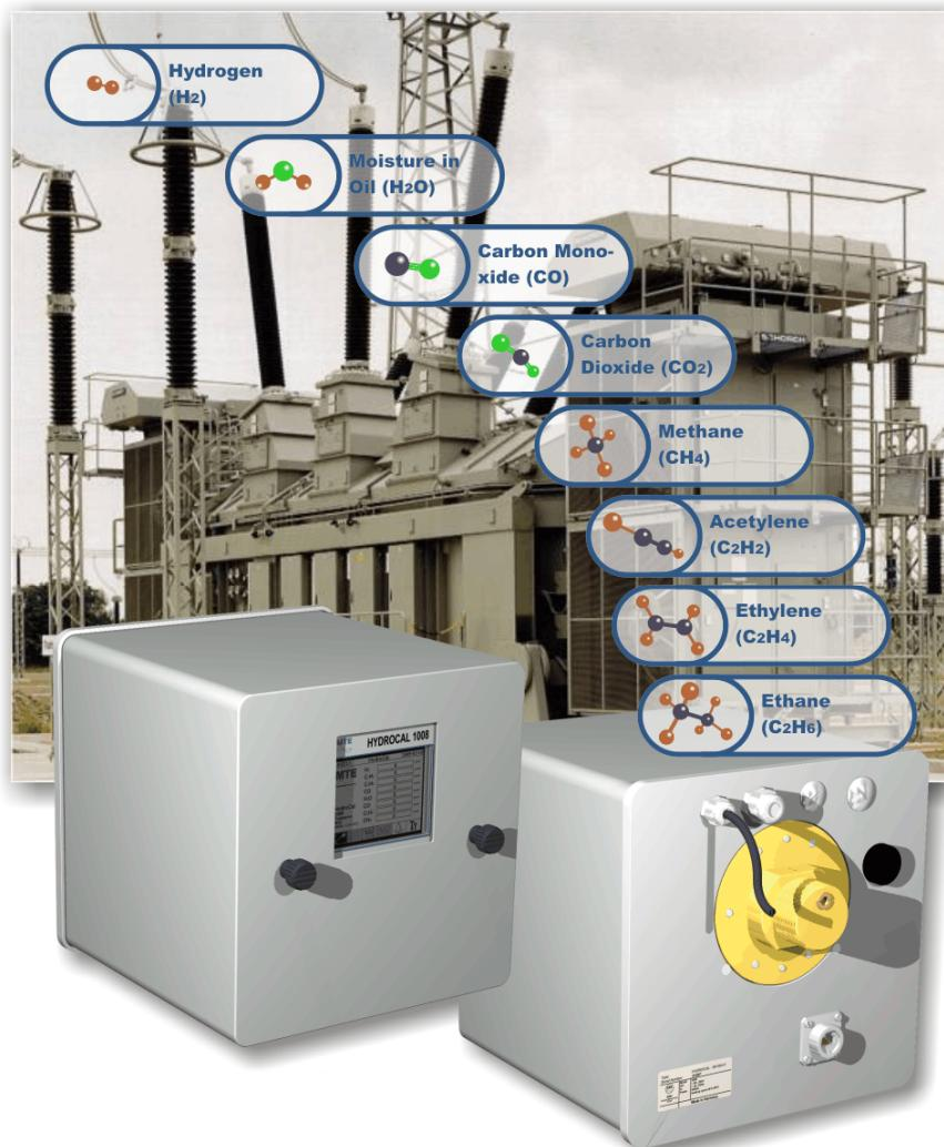
The HYDROCAL 1008 is a permanently-installed multi-gas-in-oil analysis system with transformer monitoring functions. It allows for the individual measurement of moisture and the key gases hydrogen ( $H_2$ ), carbon monoxide (CO), carbon dioxide ( $CO_2$ ), methane ( $CH_4$ ), acetylene ( $C_2H_2$ ), ethylene ( $C_2H_4$ ) and ethane ( $C_2H_6$ ) dissolved in transformer oil.
