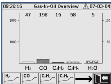
Individual chart diagram for hydrogen (H<sub>2</sub>), carbon monoxide (CO), carbon dioxide (CO<sub>2</sub>), methane (CH<sub>4</sub>), acetylene (C<sub>2</sub>H<sub>2</sub>), ethylene (C<sub>2</sub>H<sub>4</sub>) and ethane (C<sub>2</sub>H<sub>6</sub>) and moisture.
