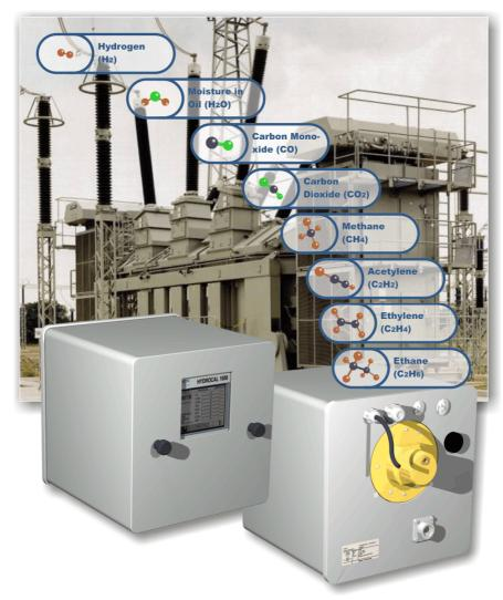
The HYDROCAL 1008 is a permanently-installed multi-gas-in-oil analysis system with transformer monitoring functions. It allows for the individual measurement of moisture and the key gases hydrogen (H<sub>2</sub>), carbon monoxide (CO), carbon dioxide (CO<sub>2</sub>), methane (CH<sub>4</sub>), acetylene (C<sub>2</sub>H<sub>2</sub>), ethylene (C<sub>2</sub>H<sub>4</sub>) and ethane (C<sub>2</sub>H<sub>6</sub>) dissolved in transformer oil.
