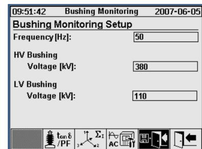
The bushing monitoring setup menu allows the input of all basic parameters required for the bushing monitoring.
