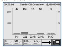
Individual chart diagram for hydrogen  $(H_2)$ , carbon monoxide (CO), acetylene  $(C_2H_2)$ , ethylene  $(C_2H_4)$  and moisture.
