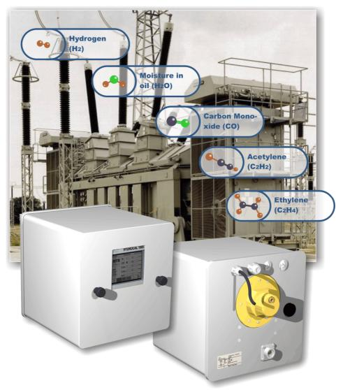
The HYDROCAL 1005 is a permanently-installed multi-gas-in-oil analysis system with transformer monitoring functions. It allows for the individual measurement of moisture and the key gases hydrogen (H<sub>2</sub>), carbon monoxide (CO), acetylene ( $C_2H_2$ ) and ethylene ( $C_2H_4$ ) dissolved in transformer oil.
